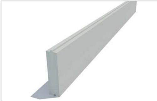
3. **“Q-CON” Wall Panel** is pre-fabricated reinforced that you can use to build interior and exterior walls. The walls that are built by Q-CON wall panels can withstand 180 Kg/sq.m. of direct wind load. It is available with 60 cm width, 6 m of maximum length, and 10-20 cm thickness in 2.5 increments.
