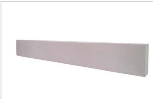
2. **“Q-CON” Lintels** is an beam with steel reinforcement that you can use horizontally above door and window frames that will support the wall built on top of it, without concrete stiffeners. Q-CON lintel comes in 10, 12.5, 15.20 cm thickness and the lengths available are from 1.2 – 3.6m in 30 cm increments.
