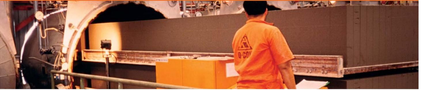
Autoclaved Aerated Concrete (AAC) is a lightweight, strong masonry product. Manufactured using naturally available materials such as sand, cement, lime, gypsum and small amounts of aluminum. And "AAC" is an energy efficient, environmentally friendly masonry product.
